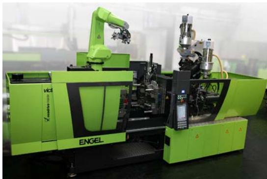
Complex hollow parts in a single step: Because the robot works inside the extended safety guarding, the production cell only requires a relatively small footprint. (Picture: ENGEL)
