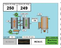
The FOCUSpro controller is an enhancement of the Focus controller – adding even more capabilities. In addition to maintaining all of the FOCUS controller's capabilities, the FOCUSpro has proportional analog capabilities.
