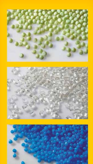
In addition to high quality, the uniform pellet size also provides for homogeneous mixture in new material. NGR thus plays an indirect role in ensuring consistent quality in the final product.
