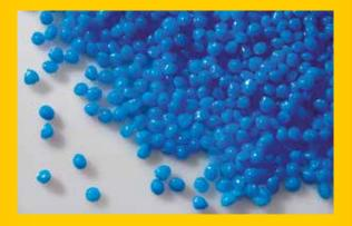
In addition to high quality, the uniform pellet size also provides for homogeneous mixture in new material. NGR thus plays an indirect role in ensuring consistent quality in the final product.
