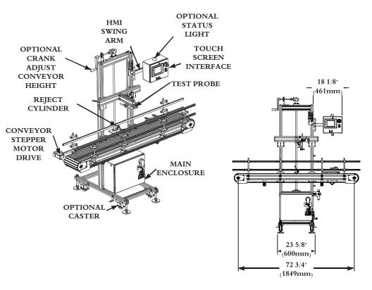
The HMI enclosure may be mounted on either side of the frame, in a position above or below the conveyor, as specified at the time of order. In the images shown above, the HMI is located in the Upper Right position. Machines can also be configured for either flow direction ("Left to Right" or "Right to Left", viewing the front of the HMI with rejects directed towards the operator).
