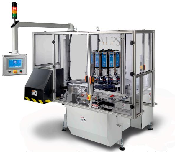
ALPS NexGen Rotary container leak inspection systems are designed to ensure production line quality through 100% inspection for the most critical defects. The system performs a functional test of the container and seal surface integrity using a pressure decay test method. Defective containers are automatically detected and ejected.
