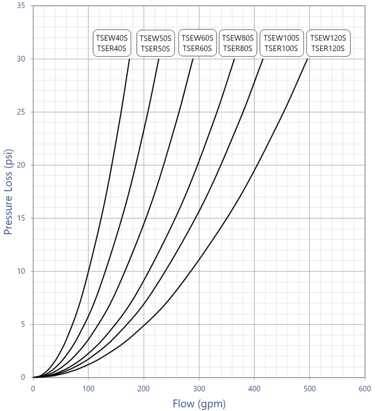
Standard Dual-Circuit Chiller Process Circuit Pressure Loss (20 to 60 Ton)
