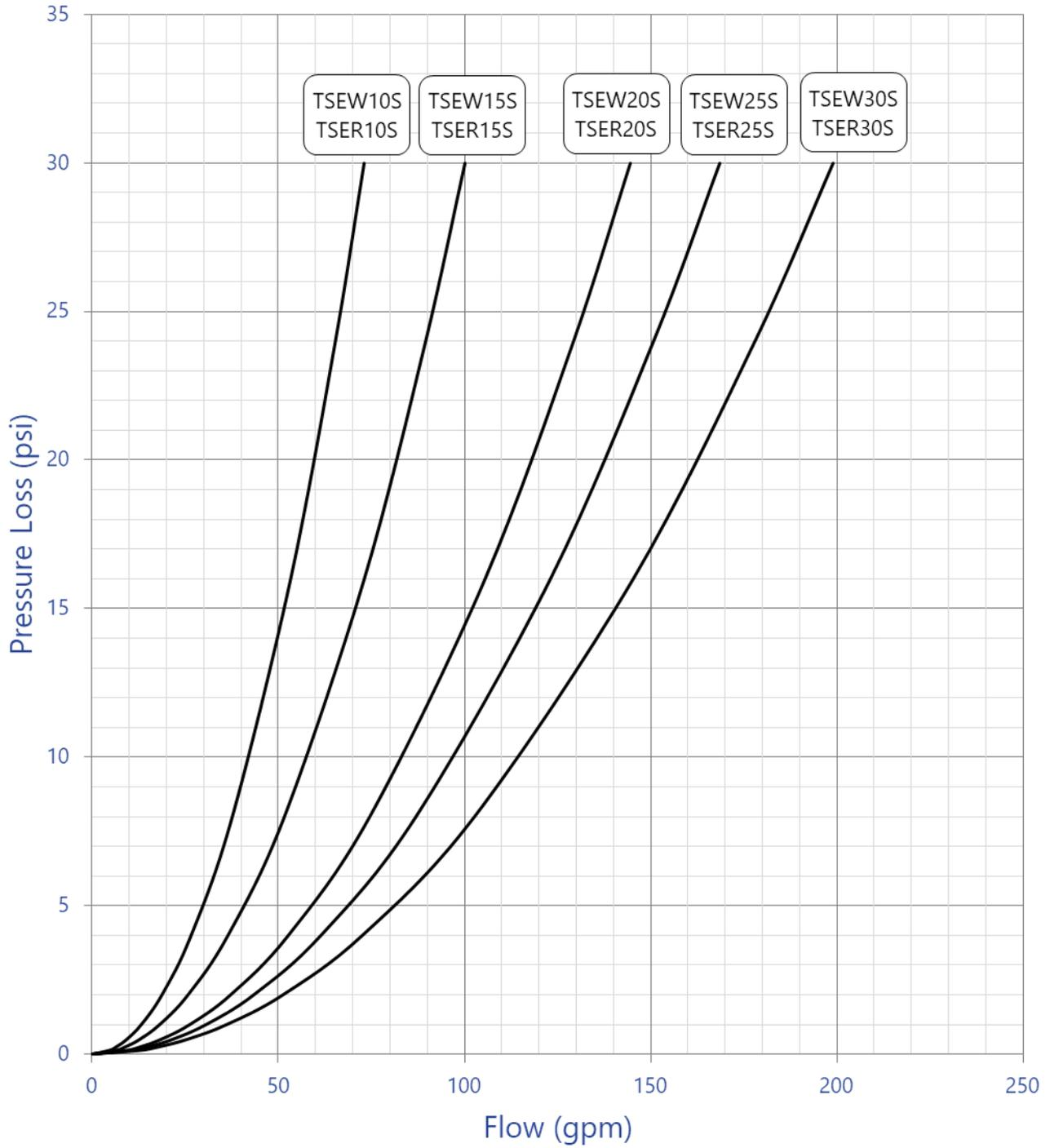
Single-Circuit Chiller with High Flow Evaporator Process Circuit Pressure Loss (40 to 120 Ton)
