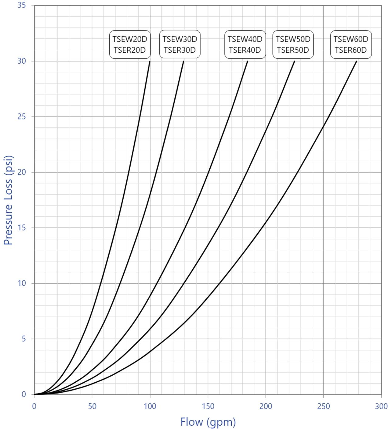
Standard Dual-Circuit Chiller Process Circuit Pressure Loss (80 to 240 Ton)
