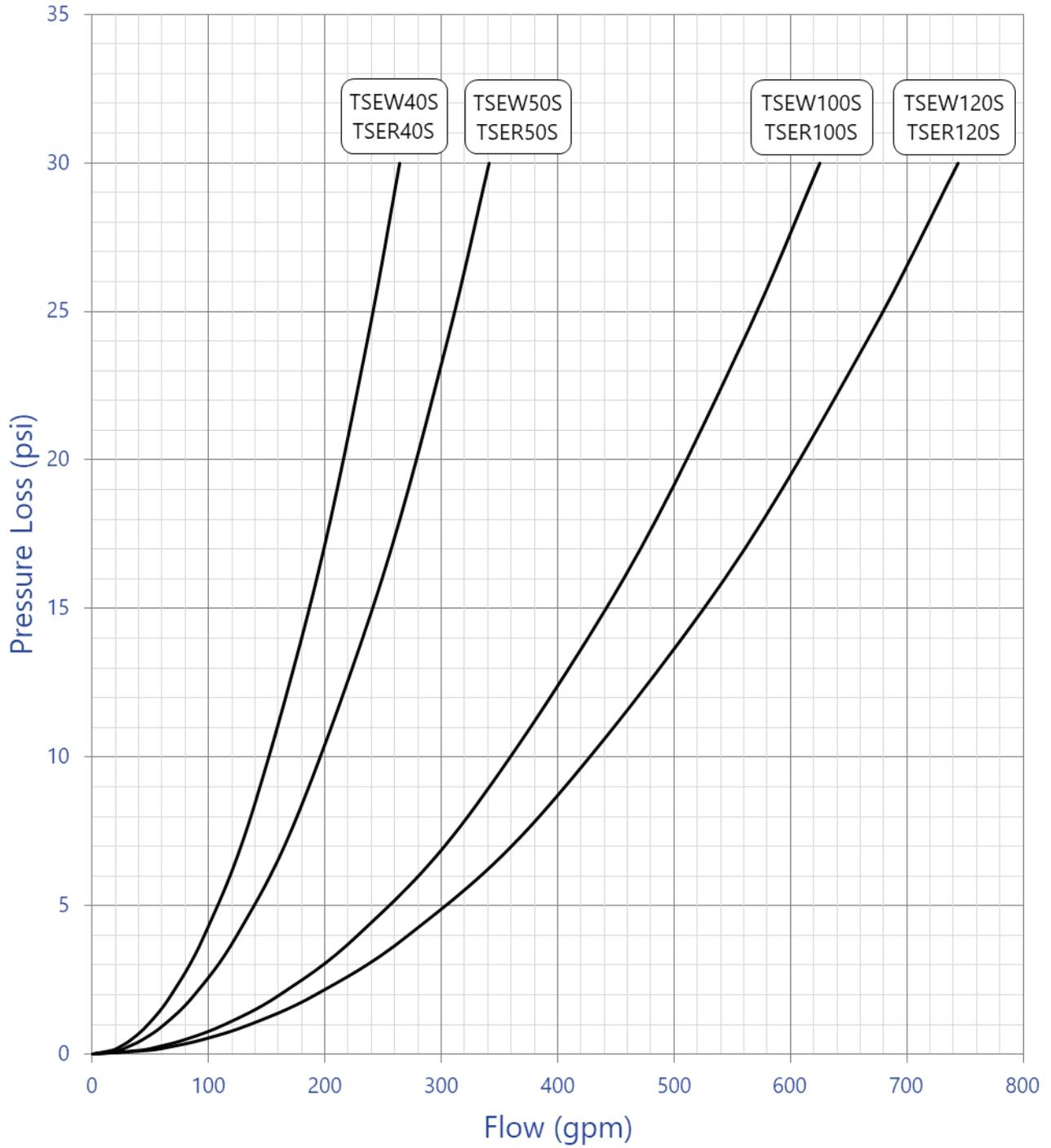
Dual-Circuit Chiller with High Flow Evaporator Process Circuit Pressure Loss (20 to 60 Ton)
