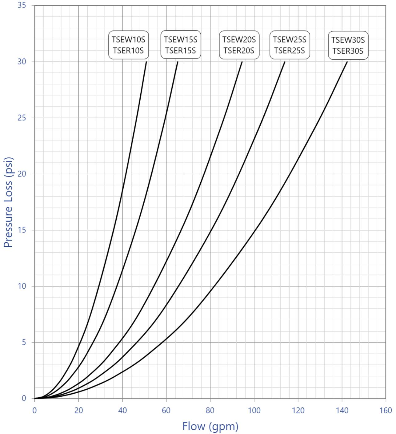
Standard Single-Circuit Chiller Process Circuit Pressure Loss (40 to 120 Ton)
