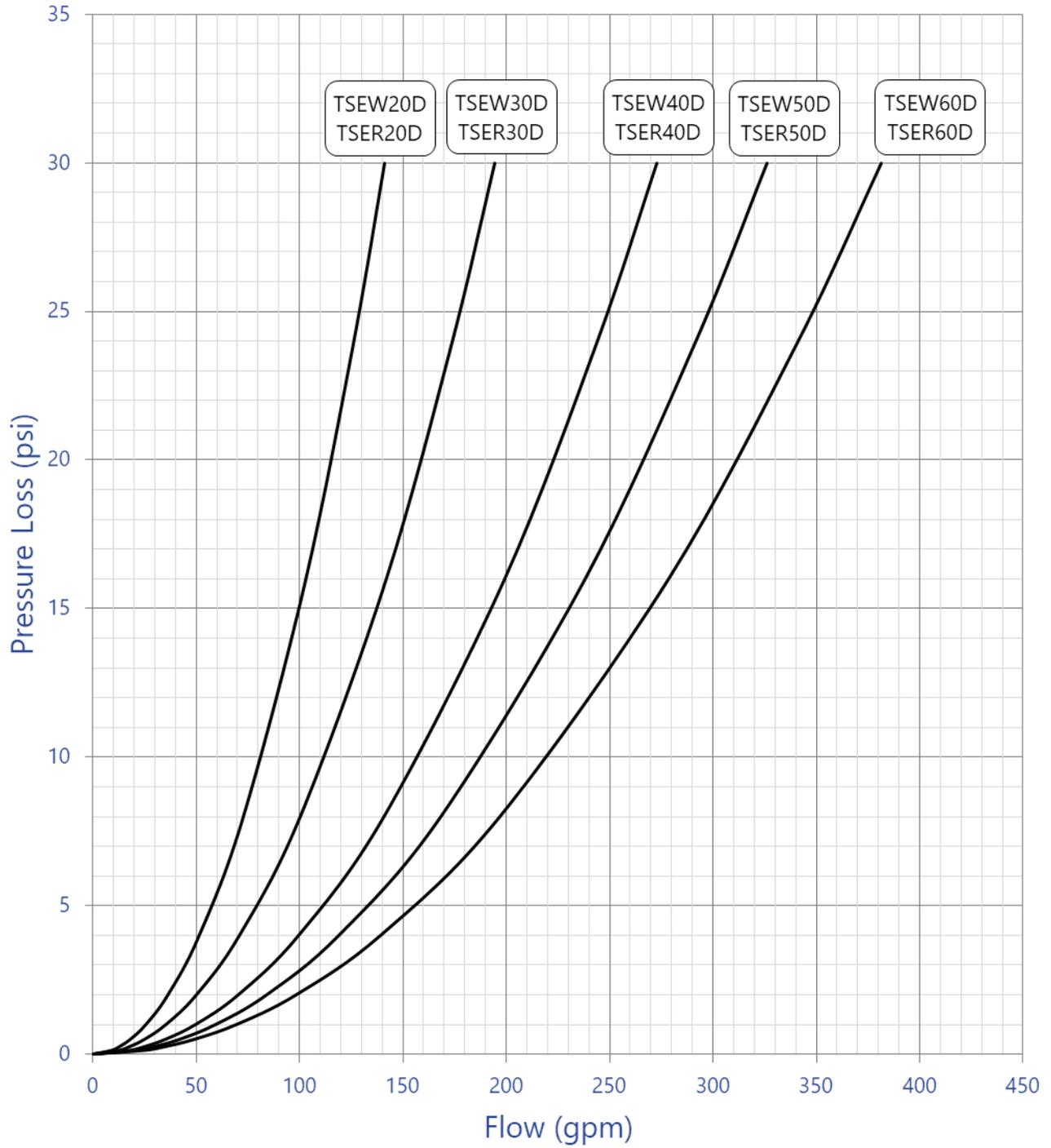
Dual-Circuit Chiller with High Flow Evaporator Process Circuit Pressure Loss (80 to 240 Ton)
