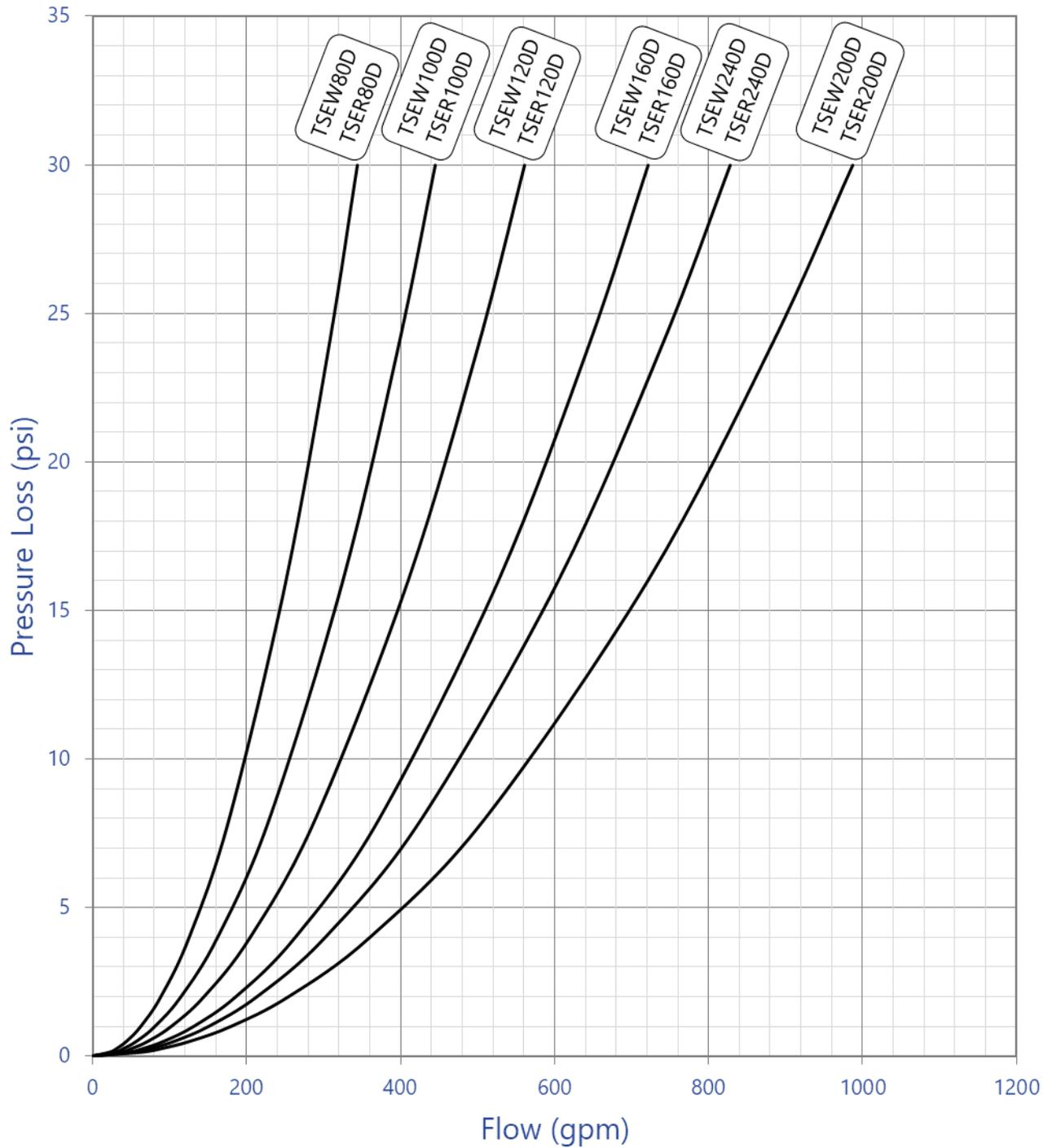
Single-Circuit Chiller with High Flow Evaporator Process Circuit Pressure Loss (10 to 30 Ton)
