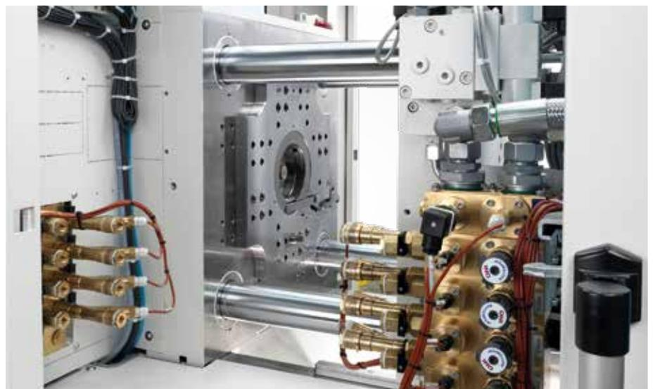
Up to 30 percent lower energy consumption by the pump of the heat-balancing units with the use of new water distributors.
