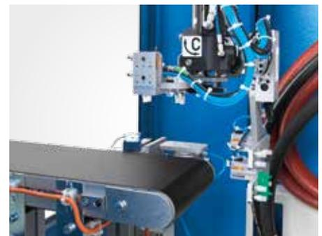
Compact conveyor belt integrated in the protective housing.
