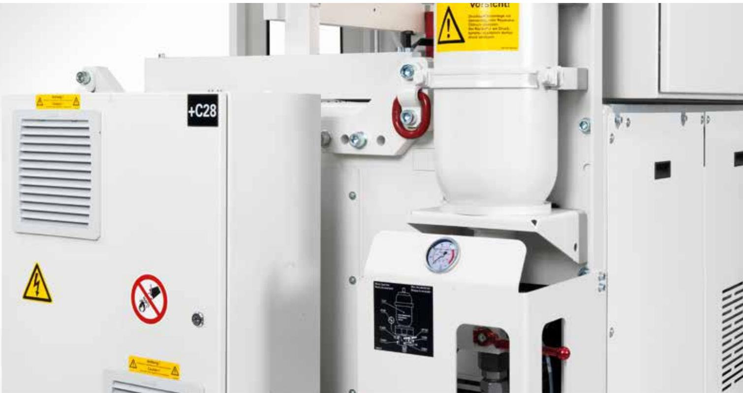
The optional BluePower Vario Drive for injection molding machines with lower clamping forces of 350 to 1,600 kN provides for low energy consumption and noise emissions.
