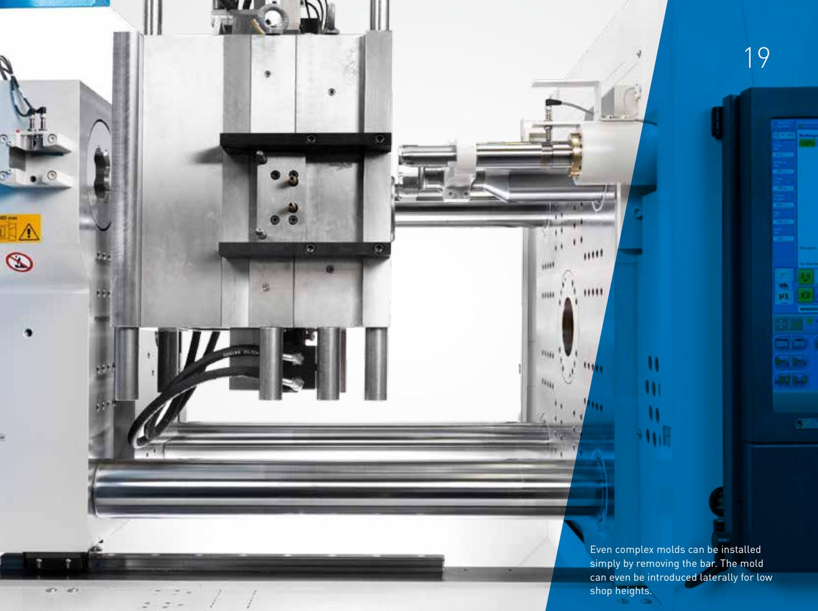
Even complex molds can be installed simply by removing the bar. The mold can even be introduced laterally for low shop heights.
