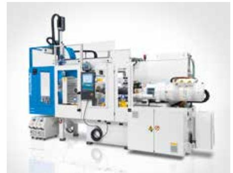
Linear robot with discharge in lengthwise direction: Parts set down on conveyor belt in standard protective housing of injection molding machine.
