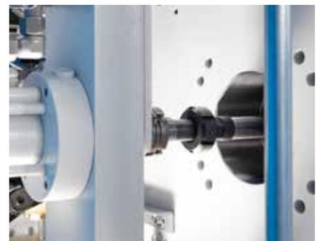
Flexible ejector coupling for fast setup, also available with adapter set
