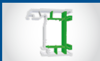
Window profiles in core technology, extruded with regrinds
