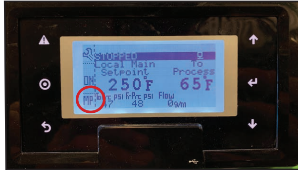
Hold "MP" Button for 3 seconds to activate mold purge.
