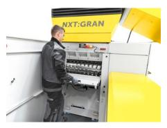
**SHREDDER KNIVES** The entire shredder cylinder with the shredder knives is freely accessible for maintenance work.
