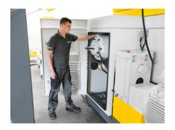
SHREDDER SHAFT The shredder shaft with its cooling water supply is protected behind a maintenance flap.
