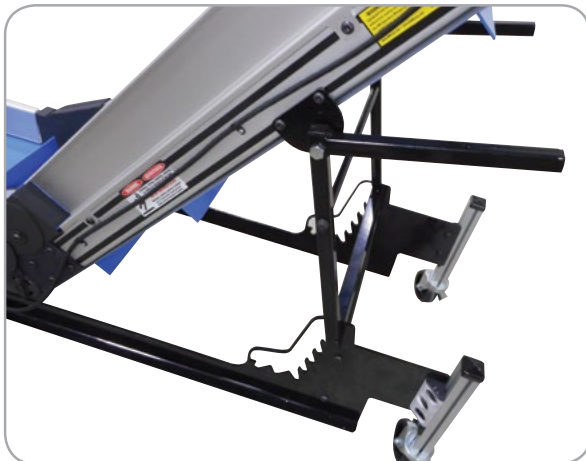
The EAK and EAZ conveyors have an optional angle adjustment rack which allows you to change the conveyor angle with no tools.
