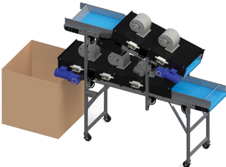
Over/Under Boxfill - EAF and EAR conveyors with two levels of cooling take up minimal floor space.
