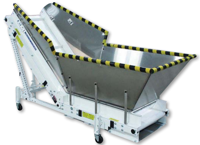
Side mounted castors allow the conveyor to sit at its lowest possible height, butting against the press to ensure maximum hopper reach into the press.
