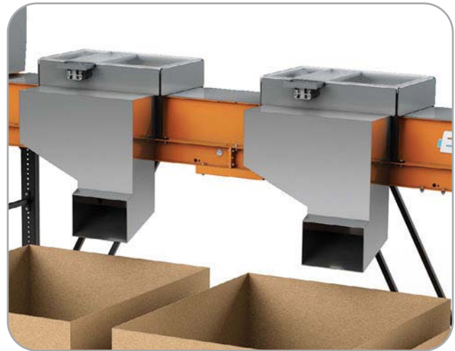
Polycarbonate enclosures and custom chutes contain parts.
