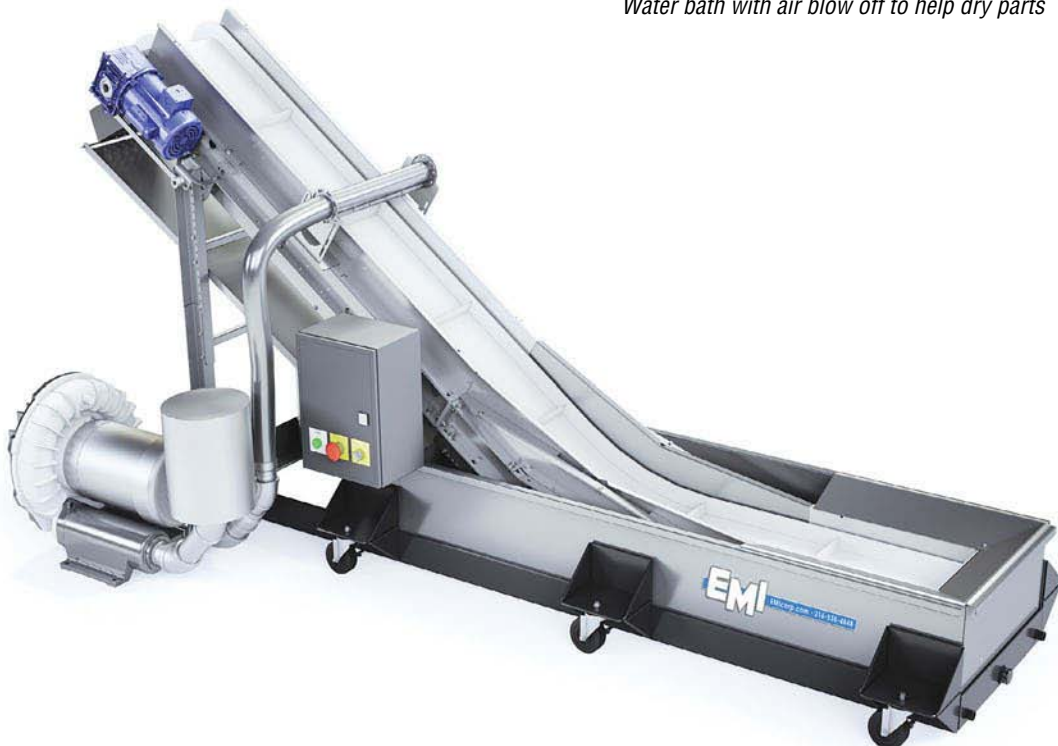
Water bath with air blow off to help dry parts
