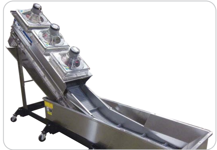
Water bath with air blow off to help dry parts
