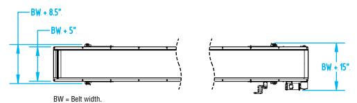
NOTE: The thickness of frame section is 7" for 51' through 180' long conveyors, 9" for 181' through 250' long conveyors.
