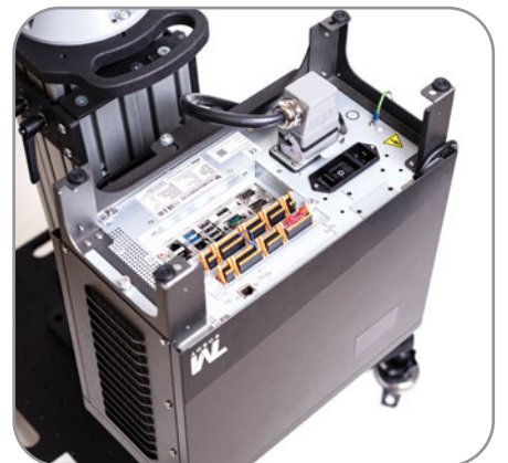
Q#8945 For Techman Control Box Mount swivels for ease of access.
