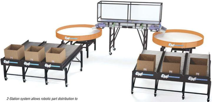
2-Station system allows robotic part distribution to multiple operators who package containers on gravity roller accumulation racks. Turntables provide flexibility for operators to work at variable pace.
