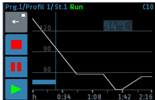
Ramp/soak programming allows for up to eight individual heating and cooling cycle programs with up to eight steps each.
